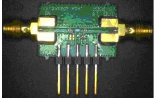
Figure 20. Evaluation/Test Board (available to qualified customer request)
