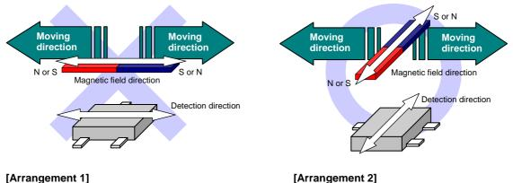
Parallel the direction of detection magnetic field with the moving direction
