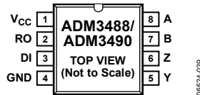
Figure 5. ADM3488/ADM3490 Pin Configuration
