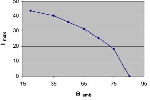
M ax. allo wable ambient Temp. at specific current (rms) B25667C3247A 175
