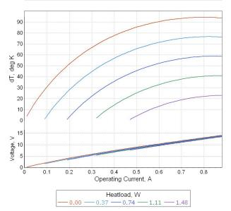
**Note**: Performance data is specified at optimal conditions (TEC hot side is stabilized at ambient temperature). Heatsink thermal resistance is not included into estimations. Use TECCad Software for estimations under different conditions.
