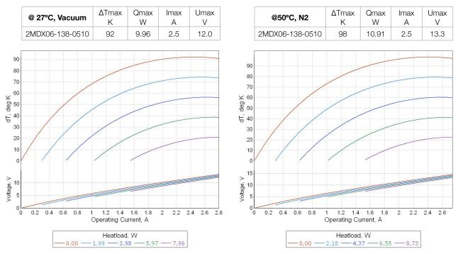
**Note**: Performance data is specified at optimal conditions (TEC hot side is stabilized at ambient temperature). Heatsink thermal resistance is not included into estimations. Use TECCad Software for estimations under different conditions.
