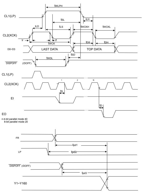
Common timing: (VSS=0V,VDD=2.5-5.5V,Vo=15 to 30v, and ta=-30 to 85°C, unless otherwise noted )
