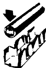
1. Prior to conductor insertion.
