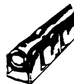
2. Insulation being pierced.
