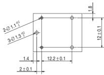
Terminal Arrangement/Internal Connections (Bottom View)
