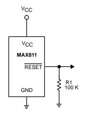
Figure 2. Ensuring RESET Valid to V<sub>CC</sub> = 0 V
