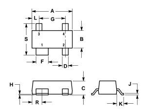
NOTES: 1. DIMENSIONING AND TOLERANCING PER ANSI Y14.5M, 1982. 2. CONTROLLING DIMENSION: MILLIMETER.
