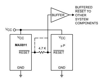
Figure 3. Interfacing to Bidirectional Reset I/O
