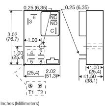
Note: Terminals 4 & 5 and/or 7 & 8 are only included on externally adjustable units.
