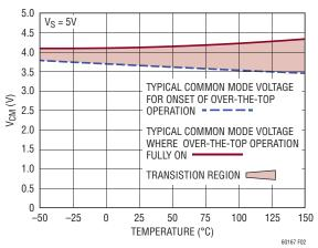
Figure 2. LT6016/LT6017 Over-The-Top Transition Region vs Temperature
