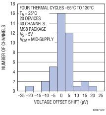
**Over-The-Top Voltage Offset vs** Temperature
