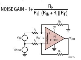
Figure 3. Difference Amplifier Configured for Both Normal and Over-The-Top Operation
