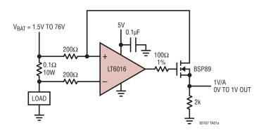
Precision High Voltage High Side Load Current Monitor
