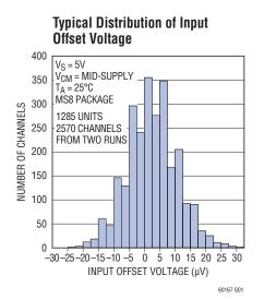
Typical Distribution of Over-The-Top Input Offset Voltage
