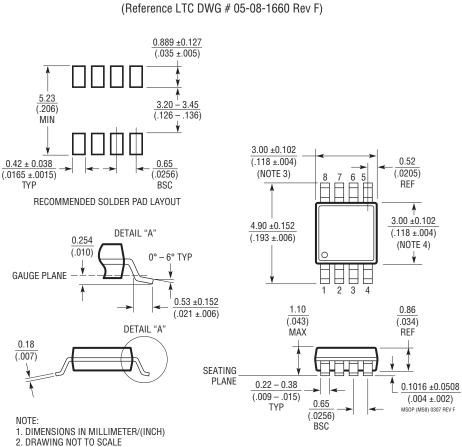
MS8 Package 8-Lead Plastic MSOP
