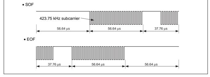
• Waveforms of SOF and EOF signals of a frame sent from a transponder (fast commands)
