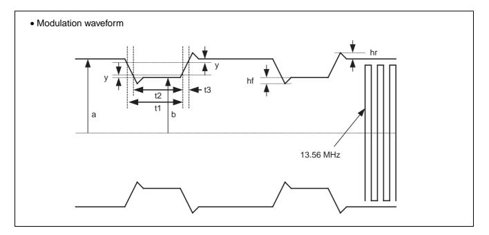
Maximum and minimum values of t1, t2 and t3 are shown in the following table. In this table, y is 0.05 (a-b) and the maximum value of hf and hr is 0.1(a-b).
