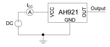
Figure 8. Test Condition of AH921 (Supply Current)
