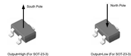
Figure 5. Output Status vs. Magnetic Pole
