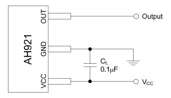
Figure 7. Test Circuit of AH921
