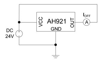
Figure 10. Test Condition of AH921 (Output Leakage Current)
