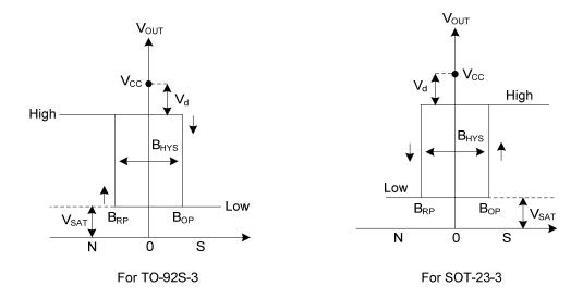
Figure 4. Magnetic Flux Density of AH921
