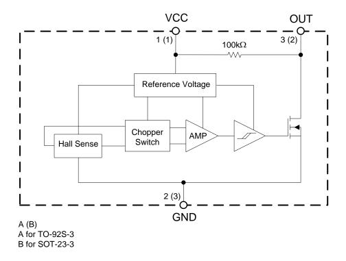
Figure 3. Functional Block Diagram of AH921
