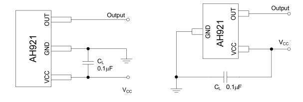
Figure 18. Typical Application Circuit of AH921
