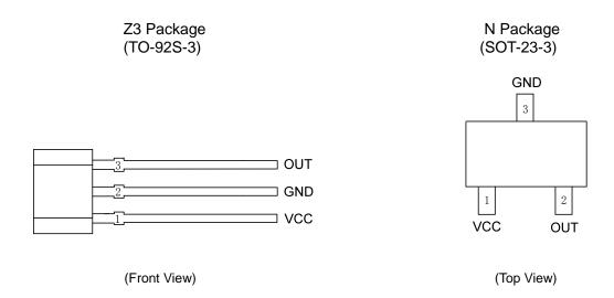
Figure 2. Pin Configuration of AH921
