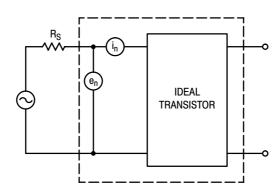
Figure 1. Transistor Noise Model
