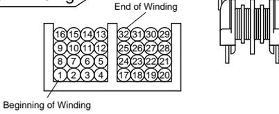
High-frequency noise can hardly pass through the Filter because both edges of coil are not close as shown above
