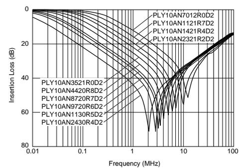
choke coil which can handle differential mode noise caused by the harmonics currents regulation circuit as well as common mode noise. It can handle noise problems much more compactly than a combination of a conventional common mode choke coil and a differential mode choke coil.
