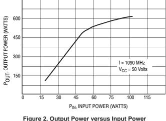
Figure 2. Output Power versus Input Power
