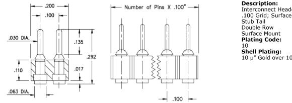
Interconnect Header .100 Grid; Surface Mount Pin Header Stub Tail Double Row Surface Mount Plating Code: 10 Shell Plating: 10 μ" Gold over 100 μ" Nickel
