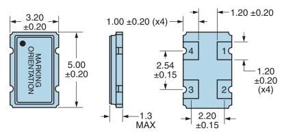
Note: Pin 1 Chamfer not shown.
