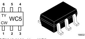
TSDF02424X Marking: WC5 Plastic case (SOT 363) 1 = Gate 1 (amplifier 1), 2 = Gate 2, 3 = Drain (amplifier 1), 4 = Drain (amplifier 2), 5 = Source, 6 = Gate1 (amplifier 2)
