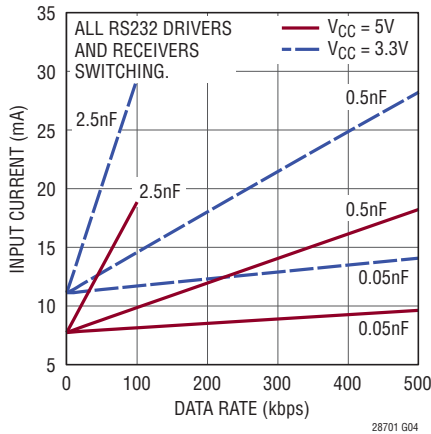
V_{CC} Supply Current vs RS232 Data Rate
