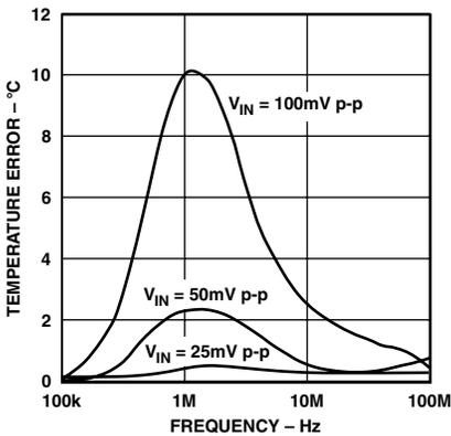
TPC 7. Temperature Error vs. Common-Mode Noise Frequency
