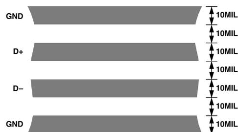
Figure 6. Arrangement of Signal Tracks
