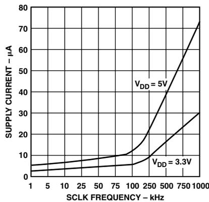
TPC 8. Standby Supply Current vs. Clock Frequency
