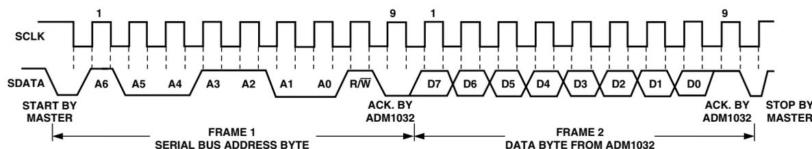
Figure 3c. Reading Data from a Previously Selected Register
