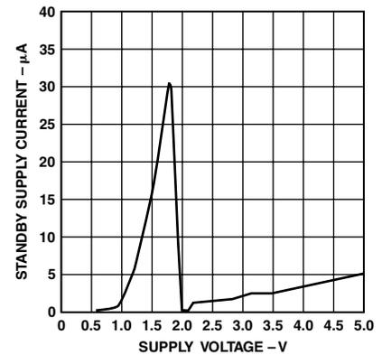
TPC 9. Standby Supply Current vs. Supply Voltage
