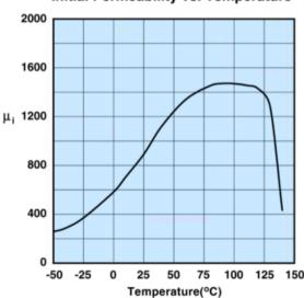
Measured on a 17/10/6mm toroid at 100kHz.
