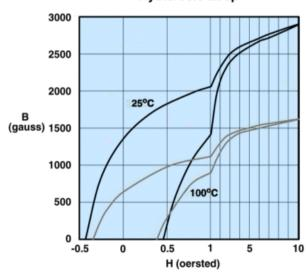
Measured on a 17/10/6mm toroid at 10kHz.
