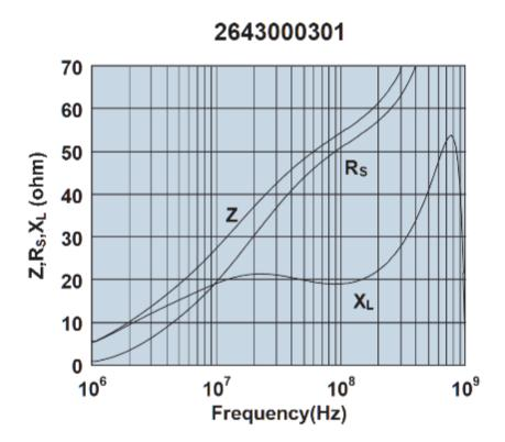
Impedance, reactance, and resistance vs. frequency.
