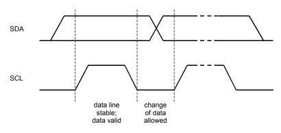
Figure 28. Bit Transfer on the I<sup>2</sup>C-Bus
