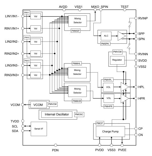
Figure 1. AK4213 Block Diagram
