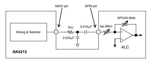
Figure 9. Example of Band-Pass-Filter for Speaker (BPF = typ. 442Hz to 4.83kHz @ -3dB)
