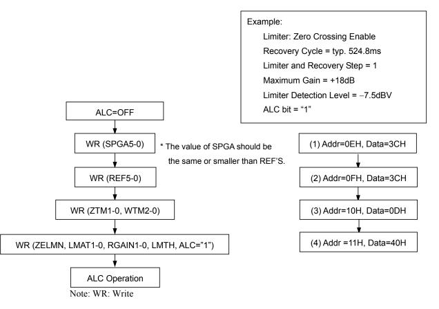
Figure 13. Registers set-up sequence at ALC operation
