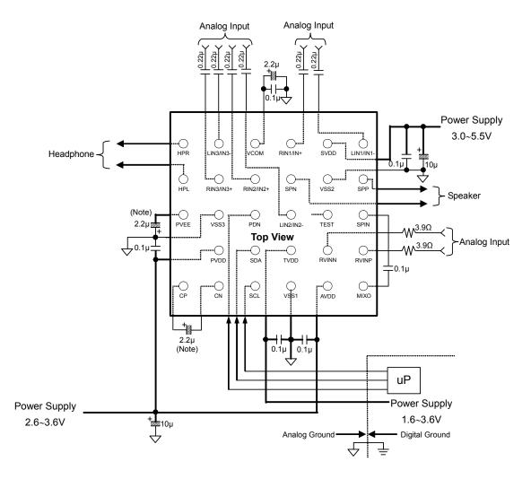
Figure 29. Typical Connection Diagram
