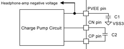
Figure 4. Charge Pump Circuit External Capacitor
