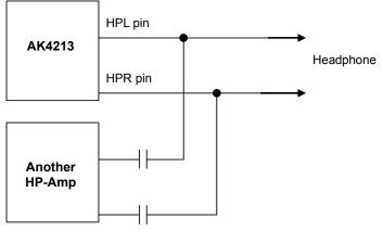
Figure 16. Wired OR with External HP-Amp
