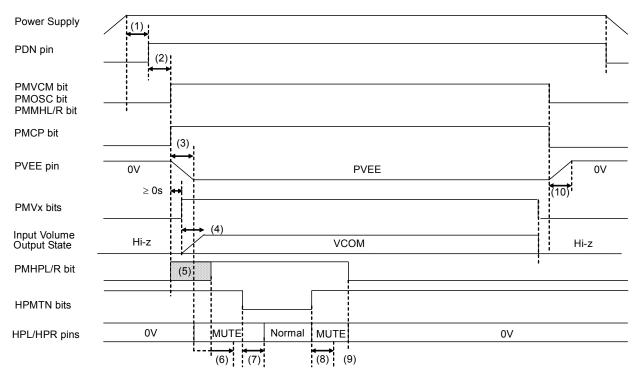
Figure 17. HP-Amp Power-up/down sequence example
