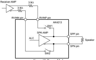
Figure 12. Bypass Mode
