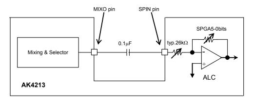
Figure 10. Example of normal connection for Speaker (fc = typ. 66Hz @ -3dB)
