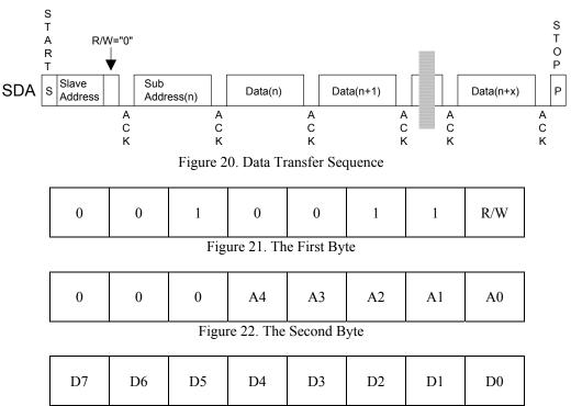
Figure 23. Byte Structure after the second byte
