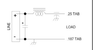
The ZA -1193-3 is an interference filter specifically designed for use in the automotive environment.
