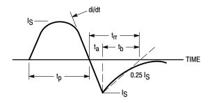
Figure 14. Diode Reverse Recovery Waveform
