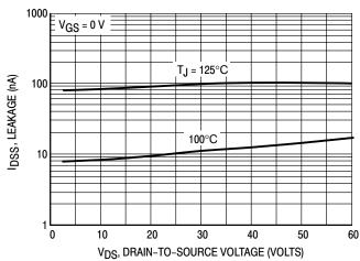
Figure 6. Drain-To-Source Leakage Current versus Voltage
