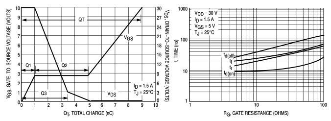
Figure 8. Gate-To-Source and Drain-To-Source
