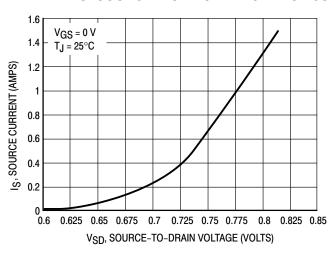
Figure 10. Diode Forward Voltage versus Current
