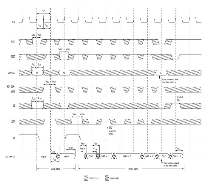
Note 22. On this diagram, when  $\overline{CE}$  is LOW:  $\overline{CE}_1$  is LOW,  $CE_2$  is HIGH, and  $\overline{CE}_3$  is LOW. When  $\overline{CE}$  is HIGH:  $\overline{CE}_1$  is HIGH,  $CE_2$  is LOW, or  $\overline{CE}_3$  is HIGH.
