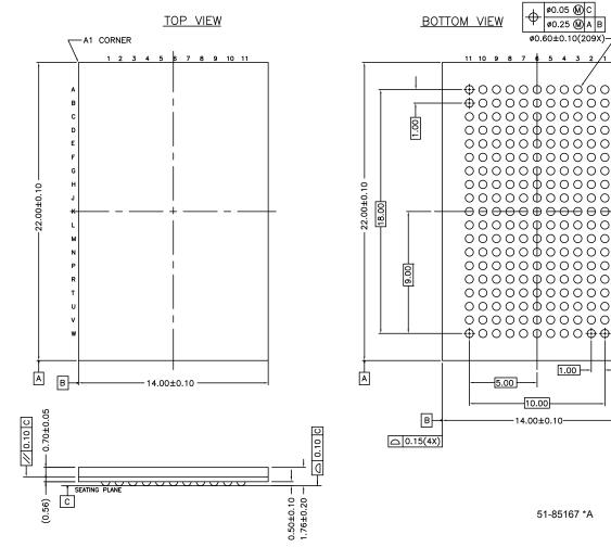
Figure 10. 209-ball FBGA (14 × 22 × 1.76 mm), 51-85167
