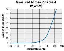
Typical Leakage vs. Temperature
