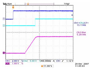
Figure 16: Turn on delay time at 12Vin, 2.5V/40A out (1mS/div) Ch1: Enable, Ch2: PG, Ch3: Vo
