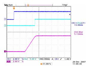
Figure 18: Turn on delay time at 12Vin, 5.0V/40A out (1mS/div) Ch1: Enable, Ch2: PG, Ch3: Vo
