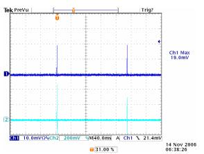
Figure 27: Short Circuit Protection at 12Vin, 1.8V out (1mS/div), Ch1: Vo, Ch2: Io, 50A/div
