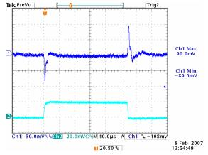
Figure 19: Transient Response at 12 Vin, 0.9V/40A out (1mS/div) Ch1: Vo, Ch2: Io, 10A/div
