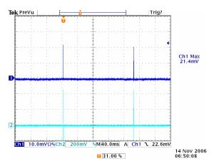
Figure 30: Short Circuit Protection at 12Vin, 5.0V out (1mS/div), Ch1: Vo, Ch2: Io, 50A/div
