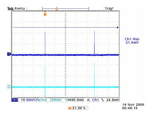
Figure 29: Short Circuit Protection at 12Vin, 3.3V out (1mS/div), Ch1: Vo, Ch2: Io, 50A/div
