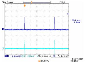
Figure 26: Short Circuit Protection at 12Vin, 1.2V out (1mS/div), Ch1: Vo, Ch2: Io, 50A/div
