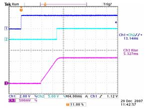
Figure 14: Turn on delay time at 12Vin, 1.2V/40A out (1mS/div) Ch1: Enable, Ch2: PG, Ch3: Vo
