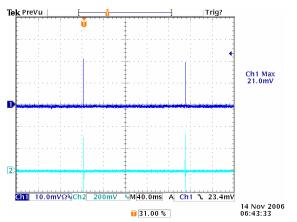
Figure 28: Short Circuit Protection at 12Vin, 2.5V out (1mS/div), Ch1: Vo, Ch2: Io, 50A/div
