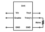
Figure 35: Trimming Output Voltage
