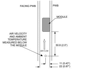
Note: Wind tunnel test setup figure dimensions are in millimeters and (Inches)
