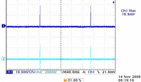
Figure 25: Short Circuit Protection at 12Vin, 0.9V out (1mS/div), Ch1: Vo, Ch2: Io, 50A/div
