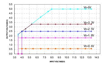
Figure 31: minimum input voltage required for output voltages above 1.8V
