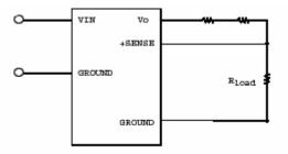
Figure 34: Circuit configuration for remote sense
