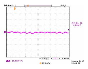
Figure 9: Output ripple & noise at 12 Vin, 1.8V/40A out (10mv/div, 2uS/div)
