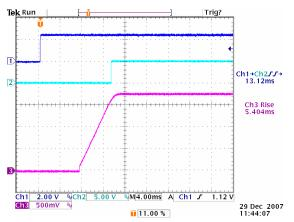
Figure 15: Turn on delay time at 12Vin, 1.8V/40A out (1mS/div) Ch1: Enable, Ch2: PG, Ch3: Vo
