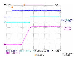
Figure 17: Turn on delay time at 12Vin, 3.3V/40A out (1mS/div) Ch1: Enable, Ch2: PG, Ch3: Vo
