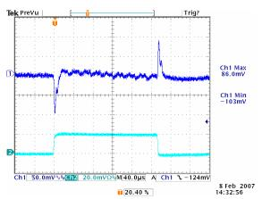
Figure 21: Transient Response at 12Vin, 1.8V/40A out (1mS/div) Ch1: Vo, Ch2: Io, 10A/div
