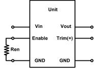
Figure 32: Enable input drive circuit example.
