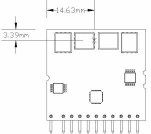
**Figure 37:** Temperature measurement location\* The allowed maximum hot spot temperature is defined at  $125 \,^{\circ}{C}$
