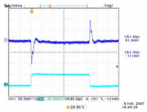
Figure 22: Transient Response at 12Vin, 2.5V/40A out (1mS/div) Ch1: Vo, Ch2: Io, 10A/div
