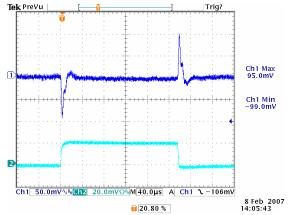
Figure 20: Transient Response at 12Vin, 1.2V/40A out (1mS/div) Ch1: Vo, Ch2: Io, 10A/div
