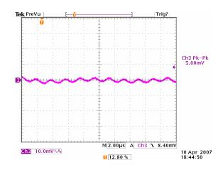
Figure 10: Output ripple & noise at 12Vin, 2.5V/40A out (10mv/div, 2uS/div)
