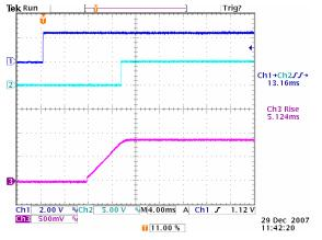
Figure 13: Turn on delay time at 12Vin, 0.9V/40A out (1mS/div) Ch1: Enable, Ch2: PG, Ch3: Vo
