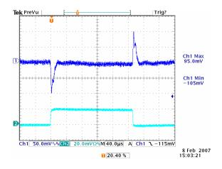
Figure 23: Transient Response at 12Vin, 3.3V/40A out (1mS/div) Ch1: Vo, Ch2: Io, 10A/div
