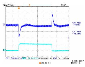
Figure 24: Transient Response at 12Vin, 5.0V/40A out (1mS/div) Ch1: Vo, Ch2: Io, 10A/div
