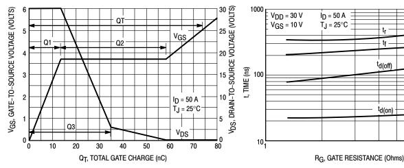
Figure 8. Gate-To-Source and Drain-To-Source **Voltage versus Total Charge**
