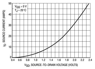
Figure 10. Diode Forward Voltage versus Current
