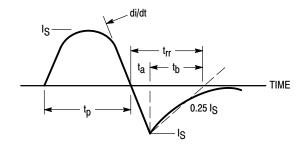
Figure 15. Diode Reverse Recovery Waveform
