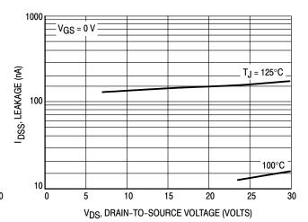
Figure 6. Drain-To-Source Leakage Current versus Voltage
