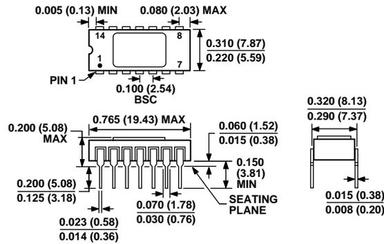
CONTROLLING DIMENSIONS ARE IN INCHES; MILLIMETER DIMENSIONS
