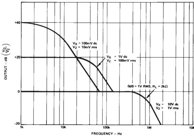
Figure 3. Frequency Response vs. Divider Denominator Input Voltage
