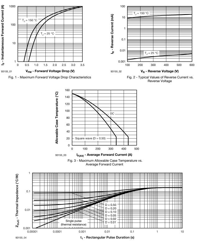
Fig. 4 - Maximum Thermal Impedance Z<sub>thJC</sub> Characteristics
