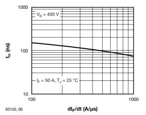
Fig. 6 - Typical Reverse Recovery Time vs. dI<sub>F</sub>/dt (Per Leg)
