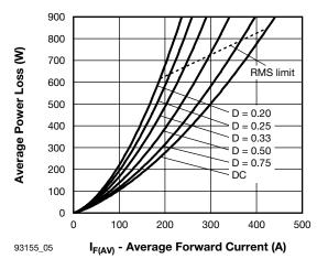
Fig. 5 - Forward Power Loss Characteristics
