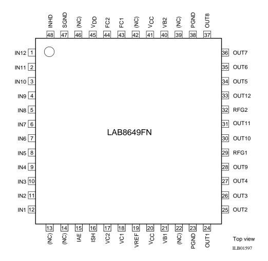
(Note) PGND is connected with both 2 pins.
