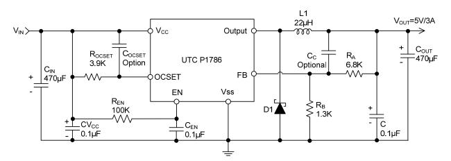
Note:  $V_{OUT}$  =  $V_{FB}$  x (1+R<sub>A</sub>/R<sub>B</sub>) , R<sub>B</sub>=0.7K~5K ohm
