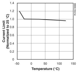
Figure 7. Current Limit vs. Temperature.
