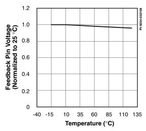
Figure 5. Feedback Pin Voltage vs. Temperature
