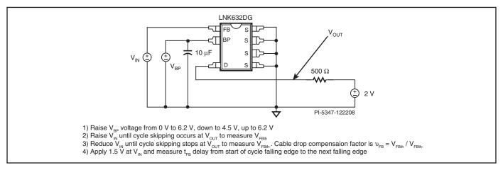
Figure 10. Test Set-up for Feedback Pin Meassurements.
