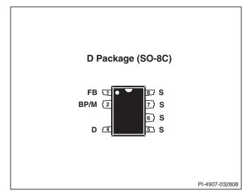
Figure 3. Pin Configuration.
