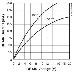
Figure 8. Output Characteristics.
