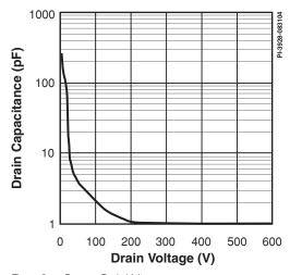
Figure 9. C<sub>oss</sub> vs. Drain Voltage.
