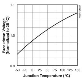
Figure 6. Breakdown vs. Temperature.
