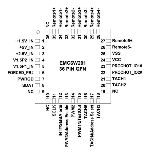
Figure 1 EMC6W201 Pin Configuration
