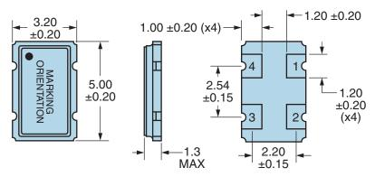
Note: Pin 1 Chamfer not shown.
