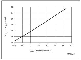
Figure 6. Drop-out voltage versus temperature.
