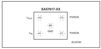
Figure 2. Pin configuration, top view (balls are on the bottom)
