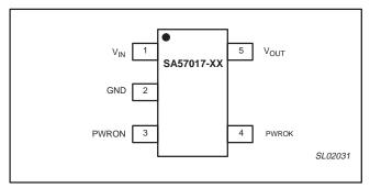
Figure 3. Pin configuration, top view
