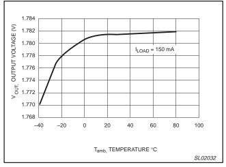
Figure 4. Output voltage versus temperature.
