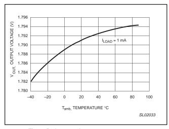
Figure 5. Output voltage versus temperature.
