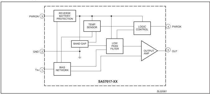
Figure 7. Simplified block diagram.
