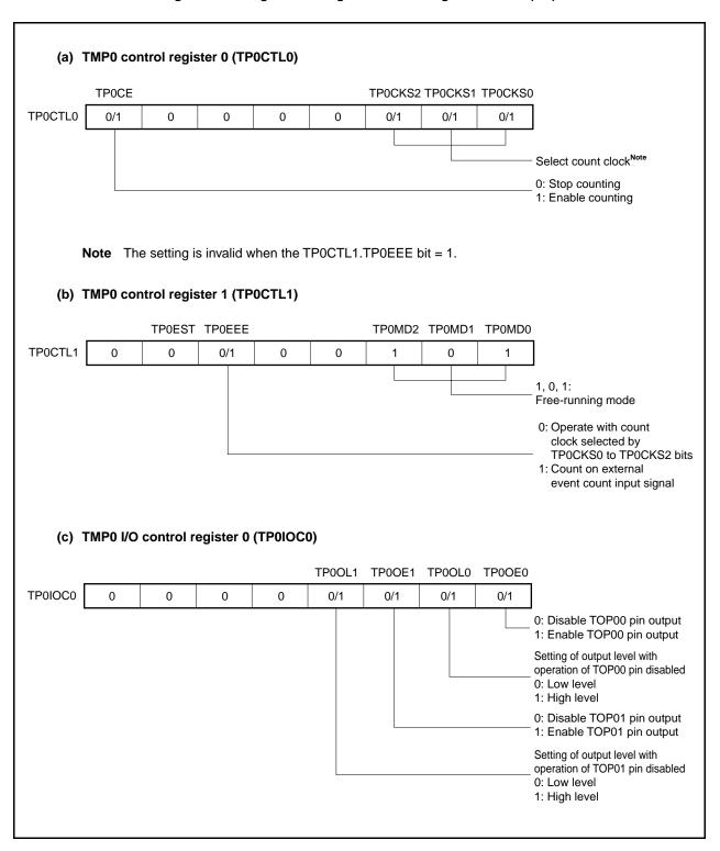
Figure 6-31. Register Setting in Free-Running Timer Mode (2/2)
