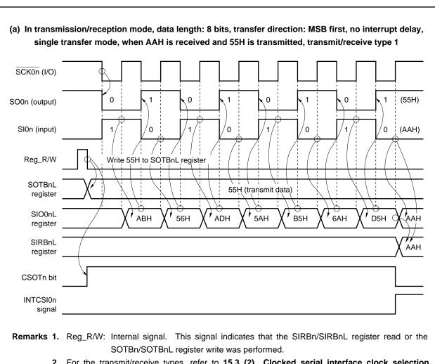
Figure 15-3. Timing Chart in Single Transfer Mode (1/2)
