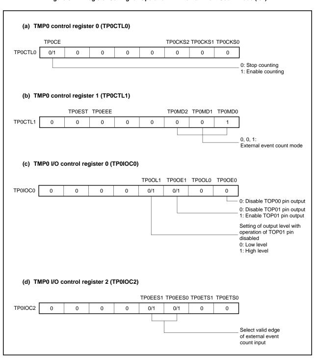
Figure 6-11. Register Setting for Operation in External Event Count Mode (2/2)
