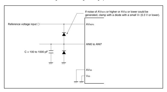
Figure 13-6. Handling of Analog Input Pins
