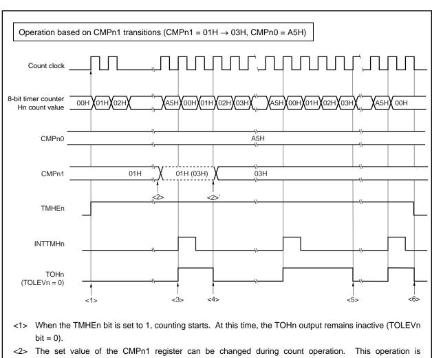
Figure 9-5. Operation Timing in PWM Output Mode (4/4)
