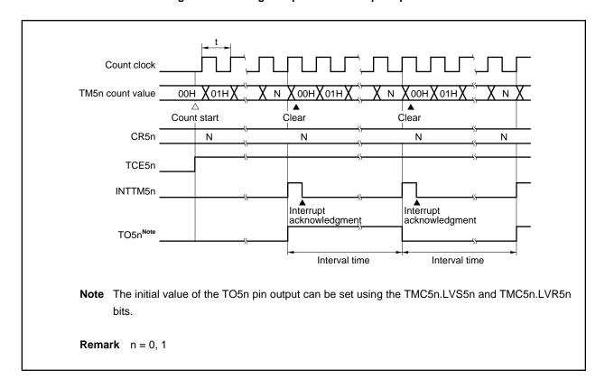
Figure 8-4. Timing of Square-Wave Output Operation
