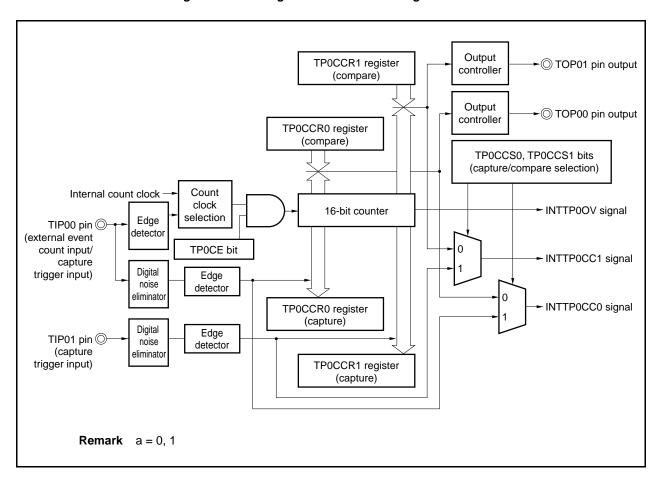
Figure 6-28. Configuration in Free-Running Timer Mode
