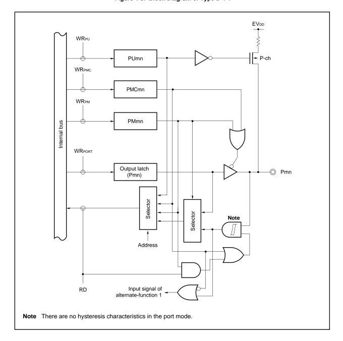
Figure 4-5. Block Diagram of Type D-1-1
