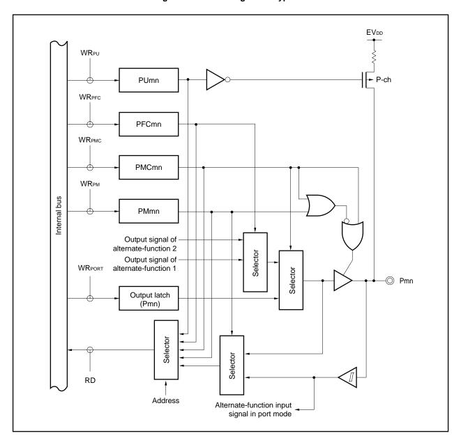
Figure 4-8. Block Diagram of Type E-4
