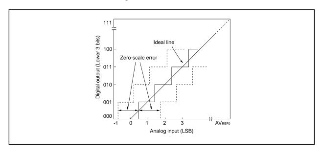
Figure 13-12. Zero-Scale Error
