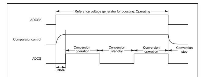
**Note** 17  $\mu$ s (14  $\mu$ s when AV<sub>REF0</sub>  $\geq$  4.0 V) or more are required for the operation of the reference voltage generator for boosting between when the ADCS2 bit is set (1) and when the ADCS bit is set (1).
