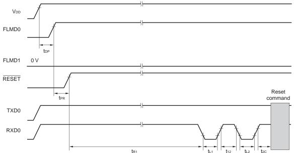
**Remark** The FLMD0 pulse does not have to be input for UART0 communication.
