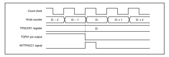
Usually, the INTTP0CC1 signal is generated when the 16-bit counter counts up next time after its count value matches the value of the TP0CCR1 register.
