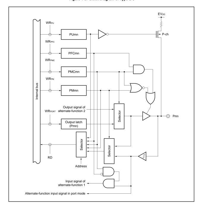
Figure 4-9. Block Diagram of Type E-5
