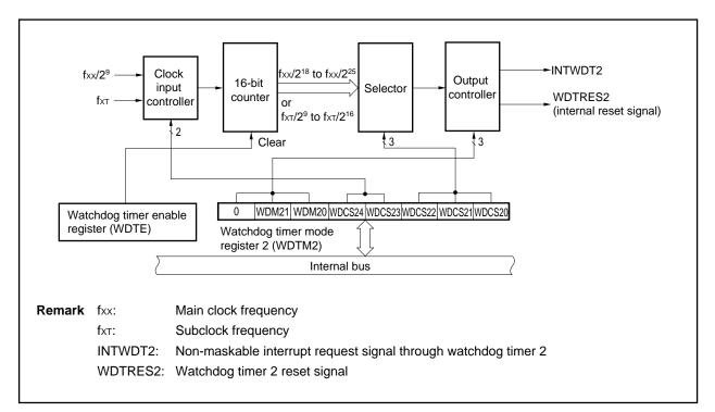
Figure 11-2. Block Diagram of Watchdog Timer 2
