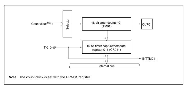
Figure 7-10. Configuration for Pulse Width Measurement with Free-Running Timer Operation
