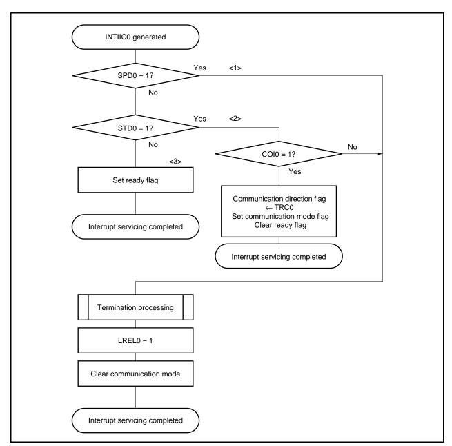
Figure 16-19. Slave Operation Flowchart (2)
