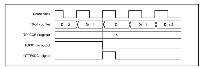
Usually, the INTTP0CC1 signal is generated in synchronization with the next counting up after the count value of the 16-bit counter matches the value of the TP0CCR1 register.
