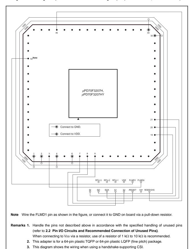
Figure 22-6. Wiring Example of V850ES/KE1 Flash Writing Adapter (FA-64GK-9ET-A, FA-64GB-8EU-A)
