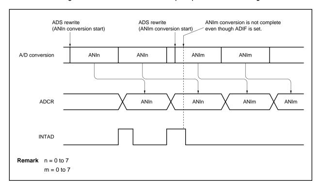
Figure 13-7. A/D Conversion End Interrupt Request Occurrence Timing
