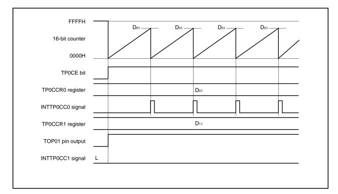
Figure 6-15. Timing Chart When D<sub>01</sub> < D<sub>11</sub>
