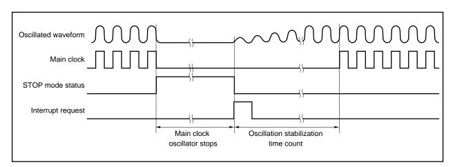
Figure 19-2. Oscillation Stabilization Time
