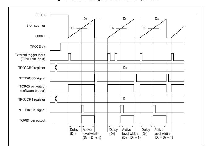
Figure 6-21. Basic Timing in One-Shot Pulse Output Mode
