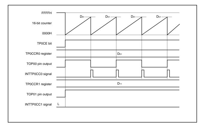
Figure 6-8. Timing Chart When D<sub>01</sub> < D<sub>11</sub>
