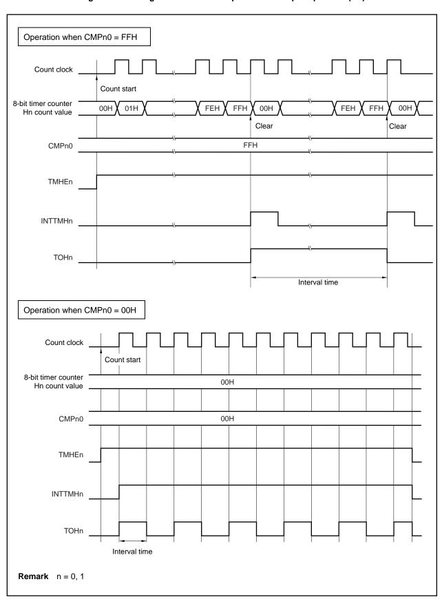
Figure 9-3. Timing of Interval Timer/Square Wave Output Operation (2/2)
