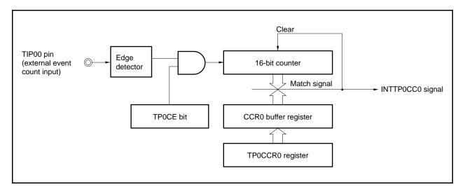
Figure 6-9. Configuration in External Event Count Mode
