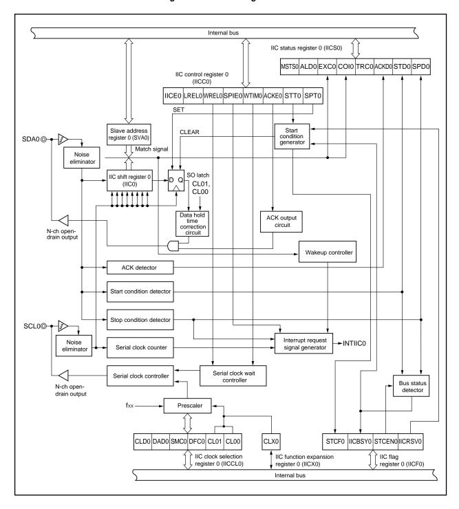
Figure 16-1. Block Diagram of I<sup>2</sup>C0
