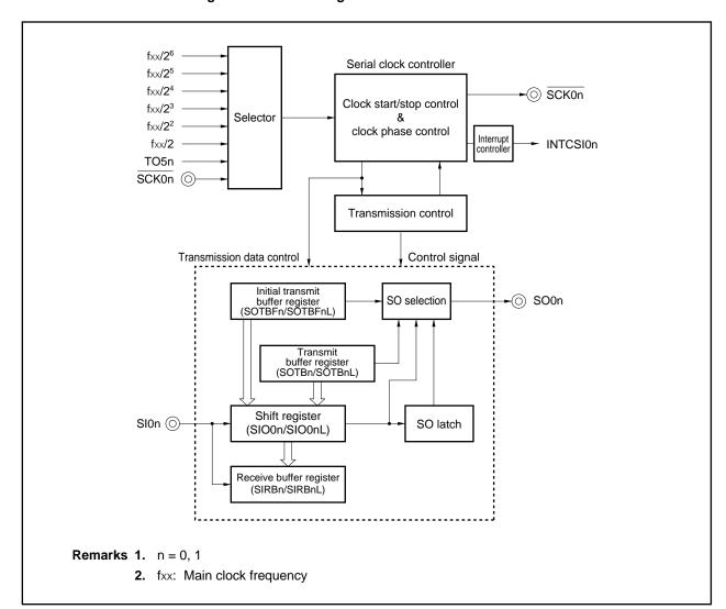
Figure 15-1. Block Diagram of Clocked Serial Interface
