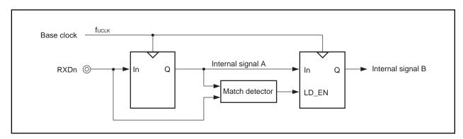
Figure 14-10. Noise Filter Circuit
