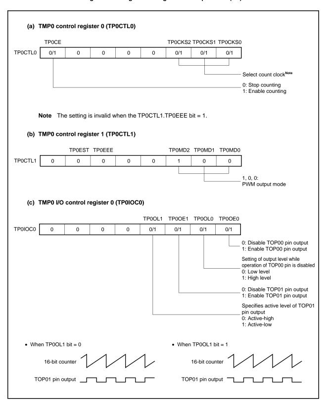
Figure 6-26. Register Setting in PWM Output Mode (2/2)
