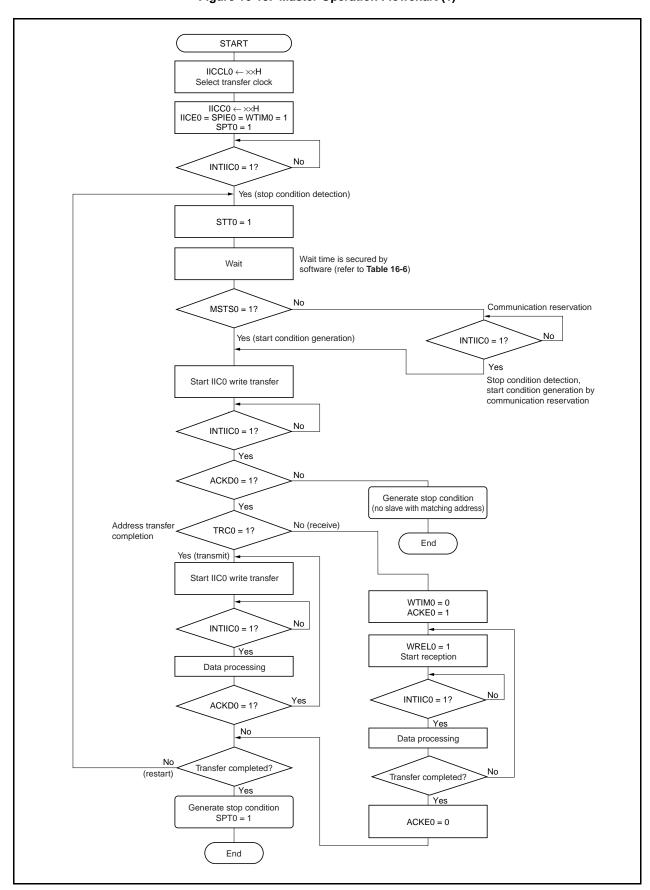
Figure 16-15. Master Operation Flowchart (1)
