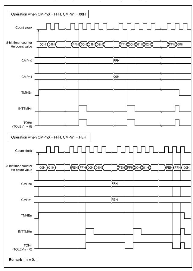
Figure 9-5. Operation Timing in PWM Output Mode (2/4)
