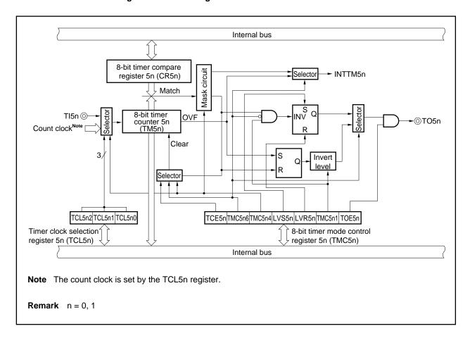
Figure 8-1. Block Diagram of 8-Bit Timer/Event Counter 5n
