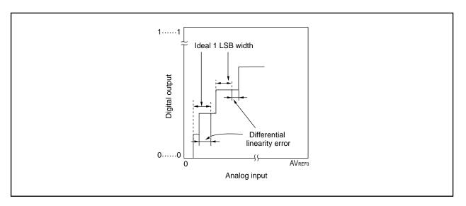
Figure 13-14. Differential Linearity Error
