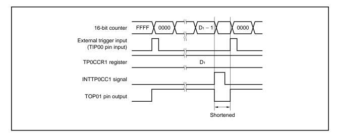
If the trigger is detected immediately before the INTTPOCC1 signal is generated, the INTTPOCC1 signal is not generated, and the 16-bit counter is cleared to 0000H and continues counting. The output signal of the TOP01 pin remains active. Consequently, the active period of the PWM waveform is extended.
