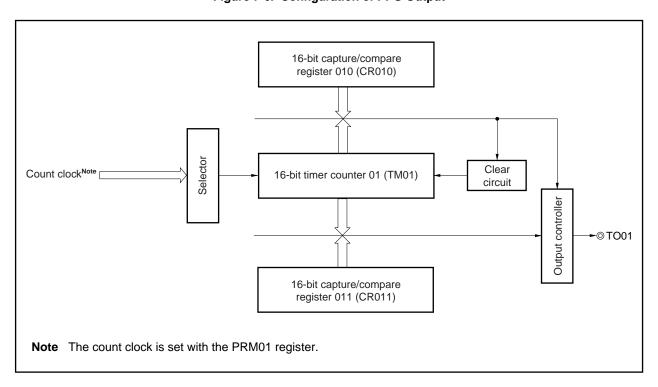
Figure 7-6. Configuration of PPG Output
