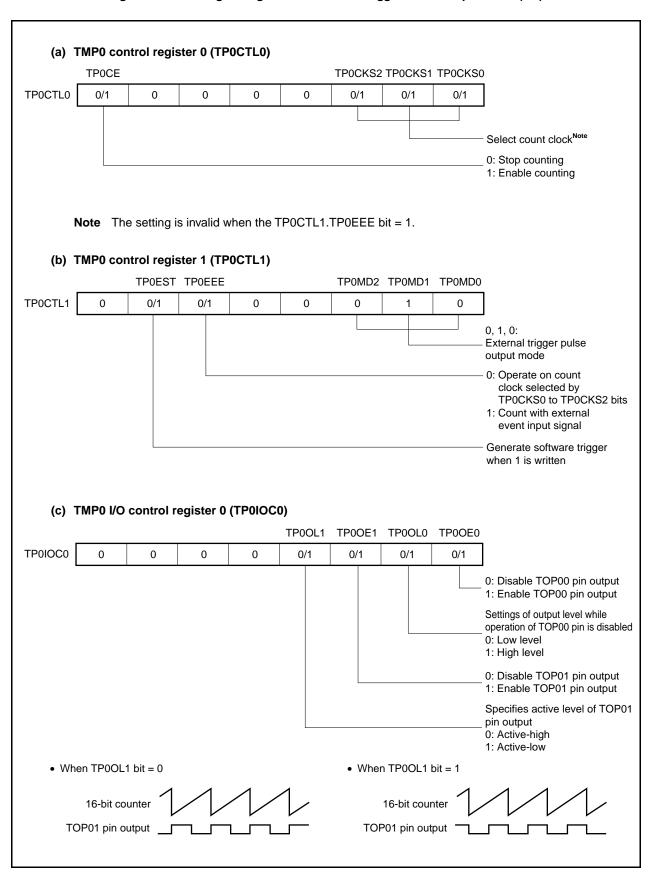
Figure 6-18. Setting of Registers in External Trigger Pulse Output Mode (2/2)
