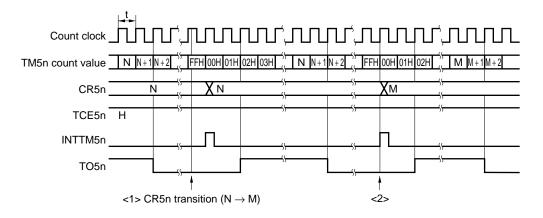
Caution In the case of read from the CR5n register between <1> and <2>, the value that is actually used differs (Read value: M; Actual value of CR5n register: N).
