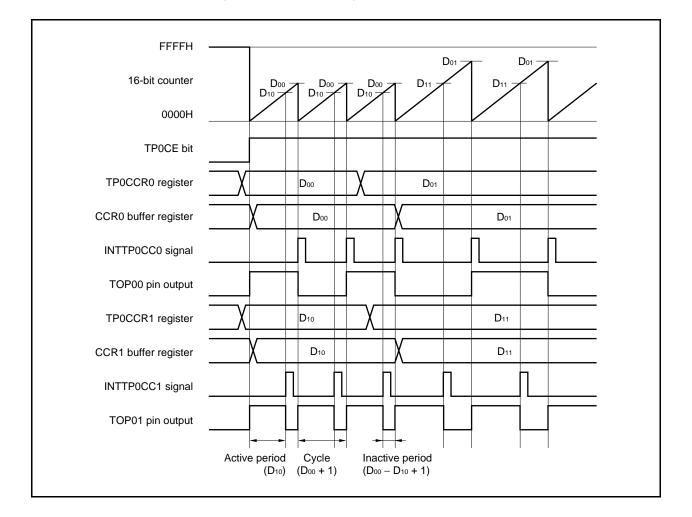
Figure 6-25. Basic Timing in PWM Output Mode
