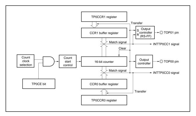
Figure 6-24. Configuration in PWM Output Mode
