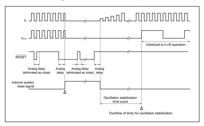
Figure 20-2. Hardware Status on RESET Pin Input
