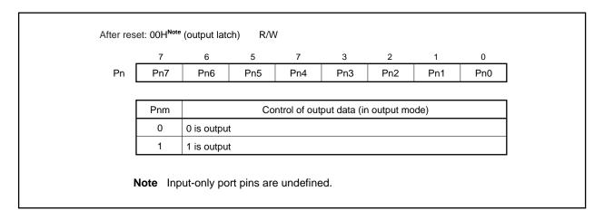
Writing to and reading from the Pn register is executed as follows independent of the setting of the PMCn register.
