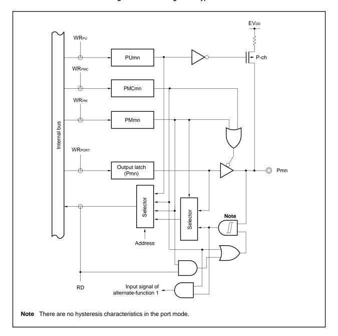
Figure 4-6. Block Diagram of Type D-1-2
