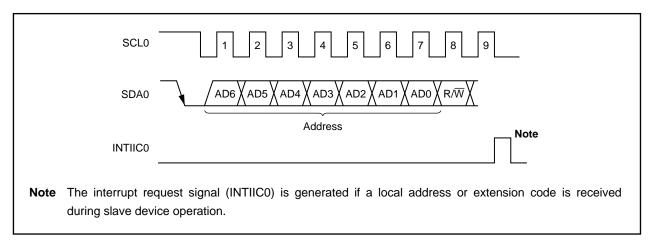
The slave address and the eighth bit, which specifies the transfer direction as described in **16.5.3 Transfer direction specification** below, are together written to the IIC0 register and are then output. Received addresses are written to the IIC0 register.
