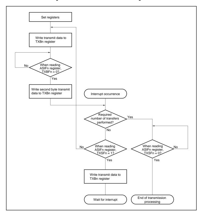
Figure 14-4. Continuous Transmission Processing Flow
