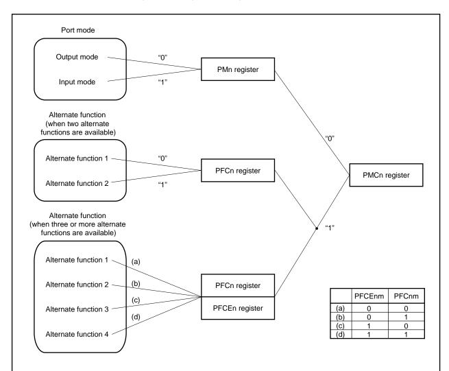
**Remark** Switch to the alternate function using the following procedure.
