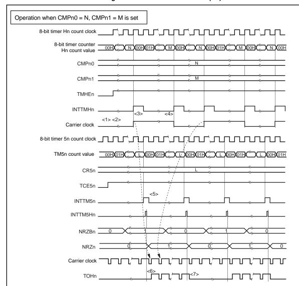
Figure 9-8. Carrier Generator Mode (2/3)
