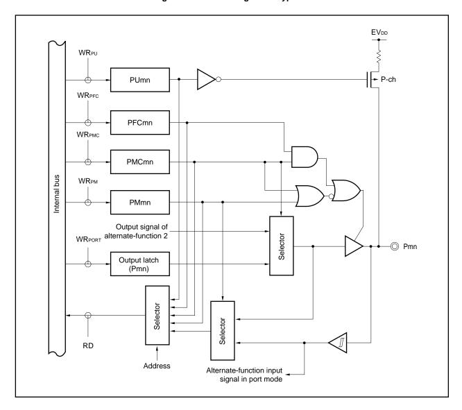
Figure 4-13. Block Diagram of Type E-9
