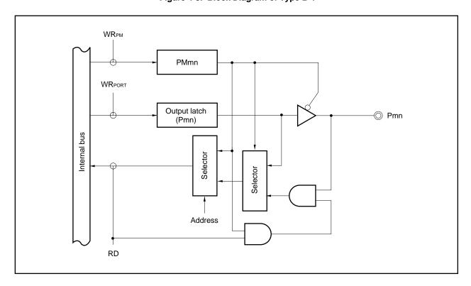
Figure 4-3. Block Diagram of Type B-1
