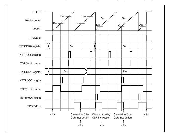
Figure 6-32. Software Processing Flow in Free-Running Timer Mode (Compare Function) (2/2)
