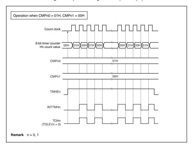
Figure 9-5. Operation Timing in PWM Output Mode (3/4)
