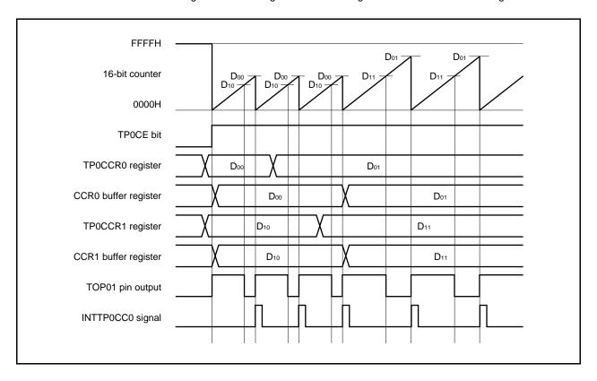
To transfer data from the TP0CCRa register to the CCRa buffer register, the TP0CCR1 register must be written.
