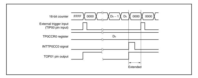
If the trigger is detected immediately before the INTTPOCC0 signal is generated, the INTTPOCC0 signal is not generated. The 16-bit counter is cleared to 0000H, the TOP01 pin is asserted, and the counter continues counting. Consequently, the inactive period of the PWM waveform is shortened.
