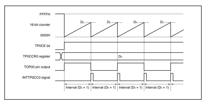
When the TP0CE bit is set to 1, the value of the 16-bit counter is cleared from FFFFH to 0000H in synchronization with the count clock, and the counter starts counting. At this time, the output of the TOP00 pin is inverted. Additionally, the set value of the TP0CCR0 register is transferred to the CCR0 buffer register.
