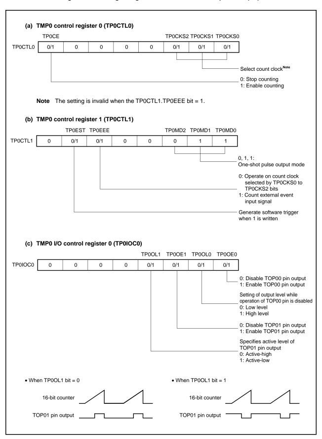
Figure 6-22. Setting of Registers in One-Shot Pulse Output Mode (2/2)
