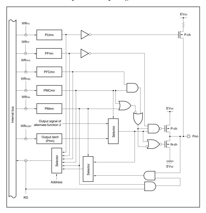
Figure 4-18. Block Diagram of Type G-9
