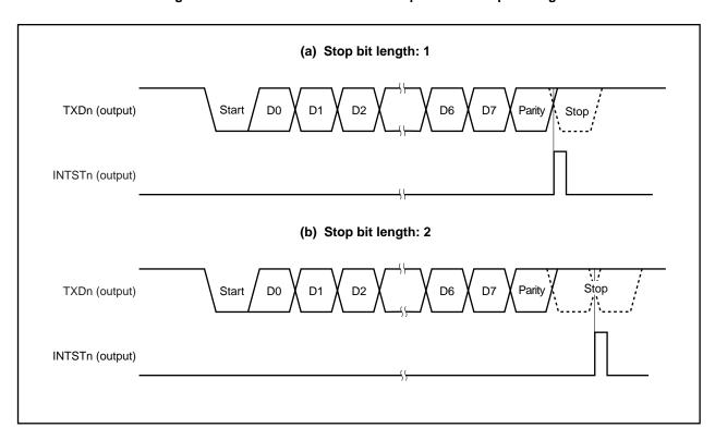
Figure 14-3. UARTn Transmission Completion Interrupt Timing
