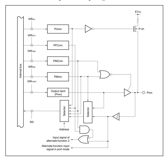
Figure 4-11. Block Diagram of Type E-7
