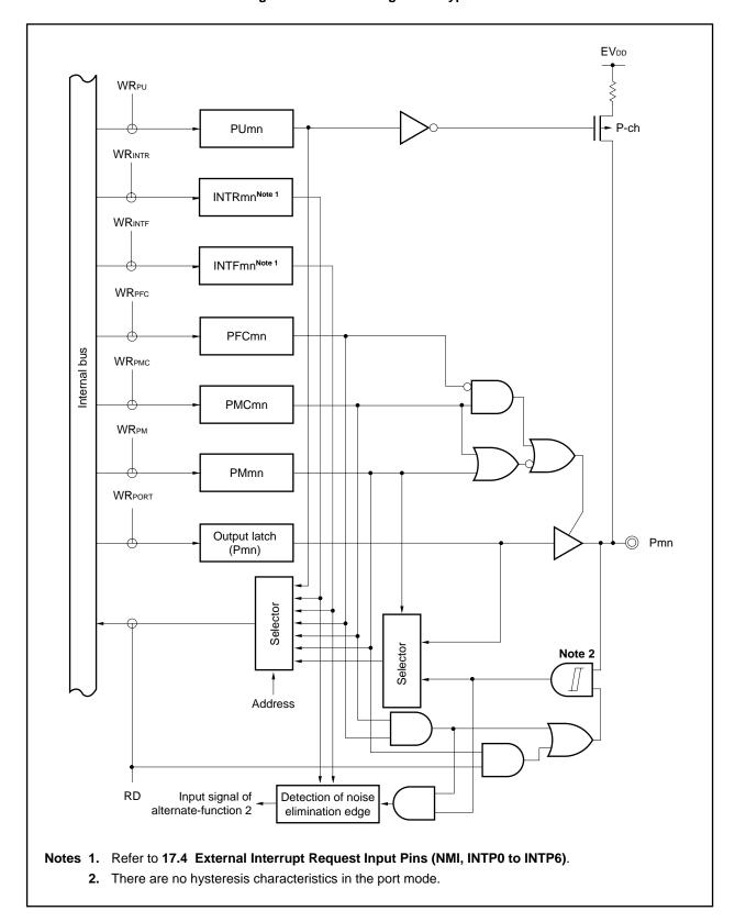
Figure 4-20. Block Diagram of Type H-3
