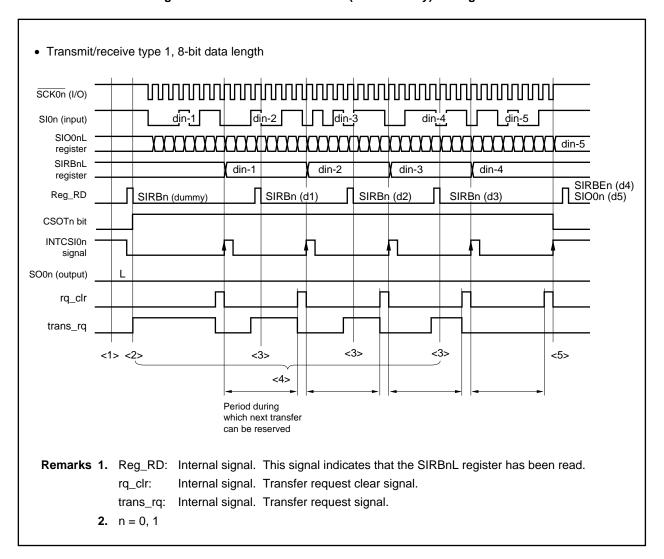
Figure 15-4. Continuous Transfer (Receive-Only) Timing Chart
