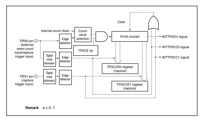
Figure 6-34. Configuration in Pulse Width Measurement Mode
