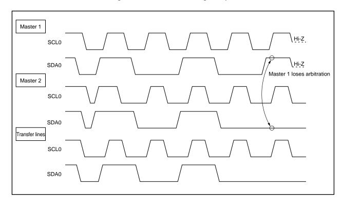
Figure 16-11. Arbitration Timing Example
