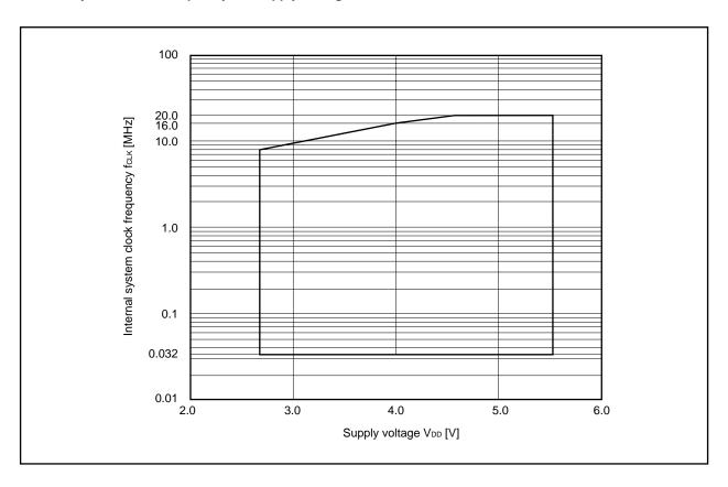
Main Clock Oscillator Characteristics (TA = -40 to +85°C, VDD = 2.7 to 5.5 V, Vss = 0 V)
