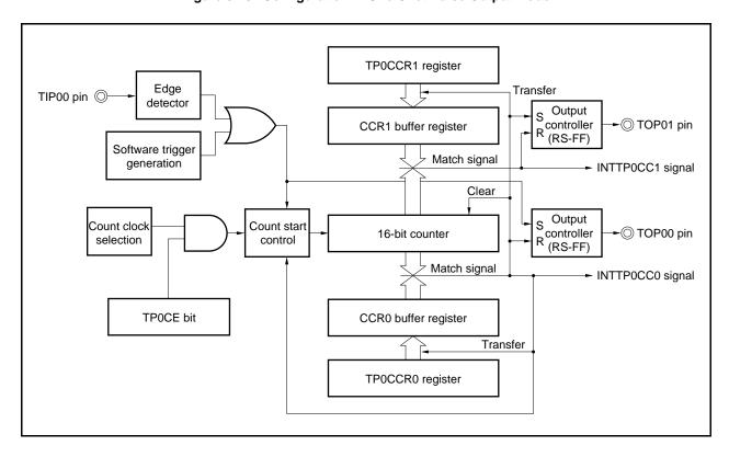
Figure 6-20. Configuration in One-Shot Pulse Output Mode
