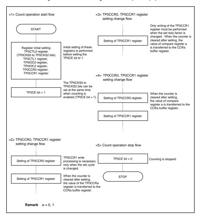
Figure 6-27. Software Processing Flow in PWM Output Mode (2/2)
