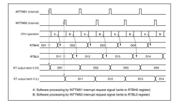
Figure 12-2. Example of Operation Timing (When EXTR0 and BYTE0 Bits = 00)
