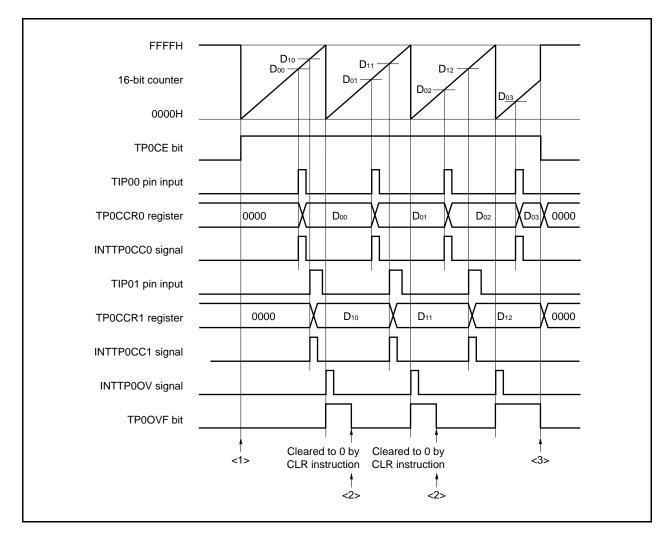
Figure 6-33. Software Processing Flow in Free-Running Timer Mode (Capture Function) (2/2)
