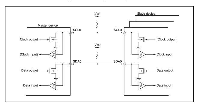
Figure 16-3. Pin Configuration Diagram
