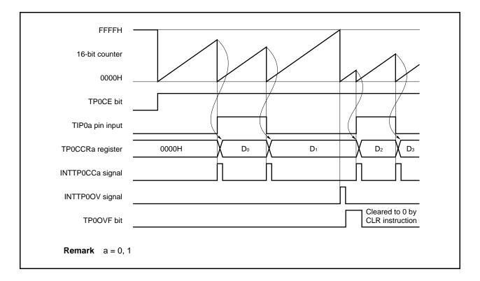
Figure 6-35. Basic Timing in Pulse Width Measurement Mode
