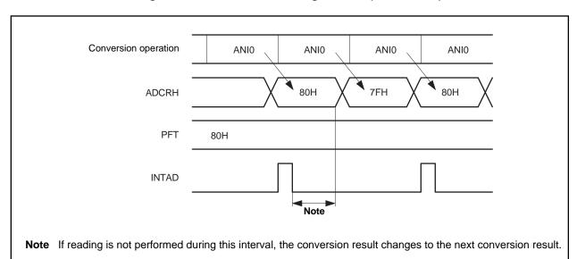
Figure 13-4. Power Fail Monitoring Function (PFCM Bit = 0)
