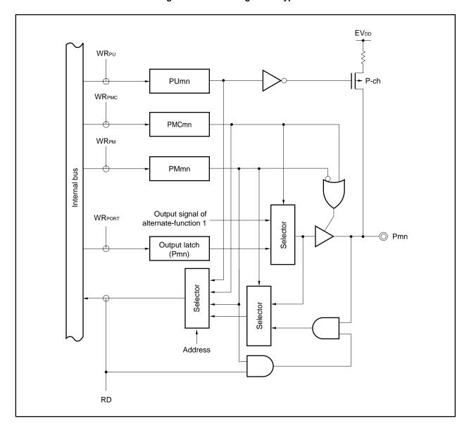
Figure 4-7. Block Diagram of Type D-2
