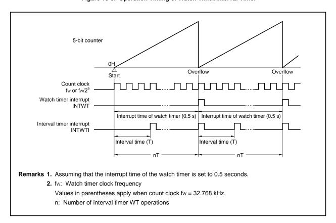
Figure 10-3. Operation Timing of Watch Timer/Interval Timer
