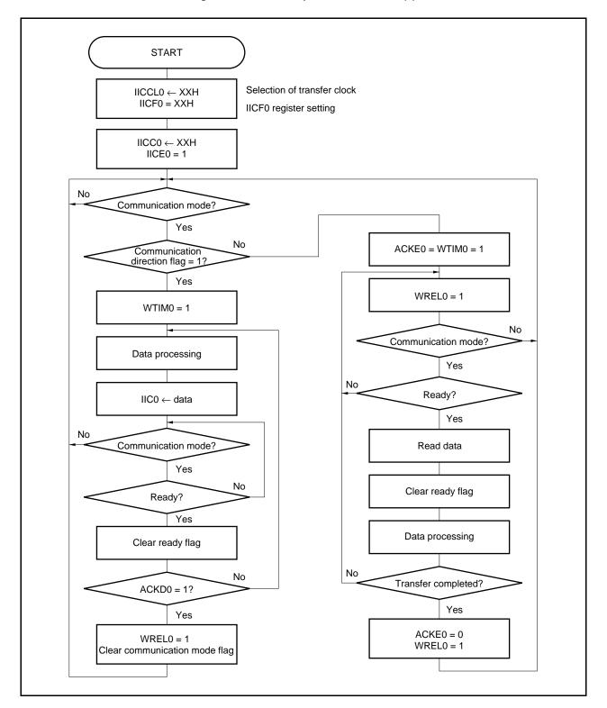
Figure 16-18. Slave Operation Flowchart (1)
