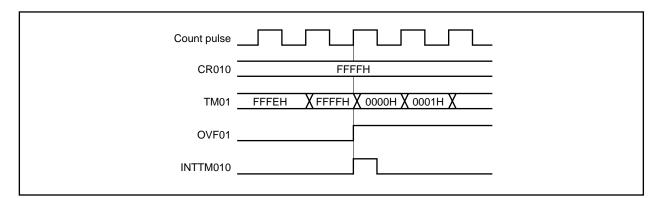
Figure 7-27. Operation Timing of OVF01 Flag
