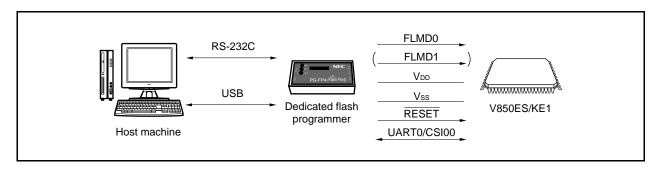
A host machine is required for controlling the dedicated flash programmer.
