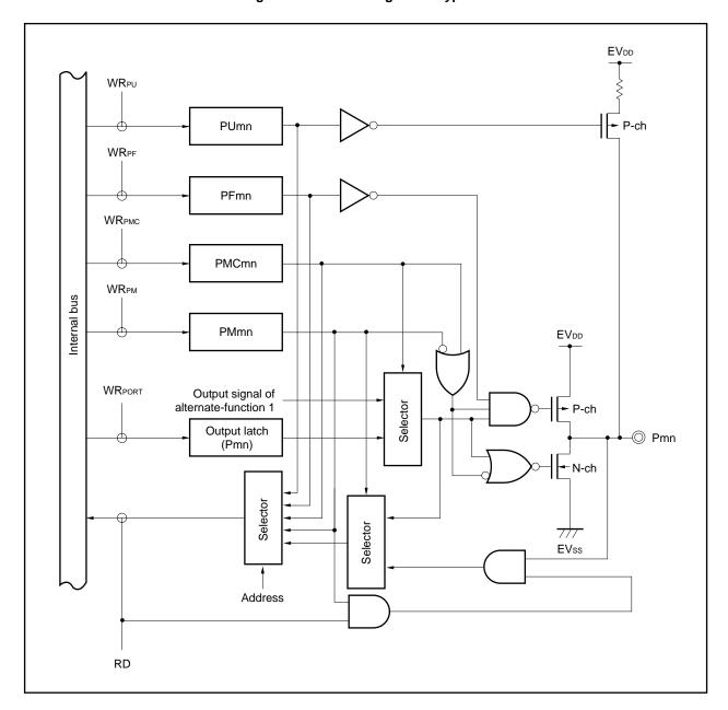
Figure 4-14. Block Diagram of Type F-1
