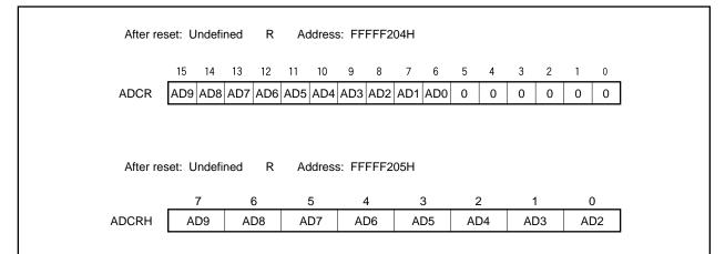
Caution When the main clock is stopped and the CPU is operating on the subclock, do not access the ADCR and ADCRH registers using an access method that causes a wait. For details, refer to 3.4.8 (2).
