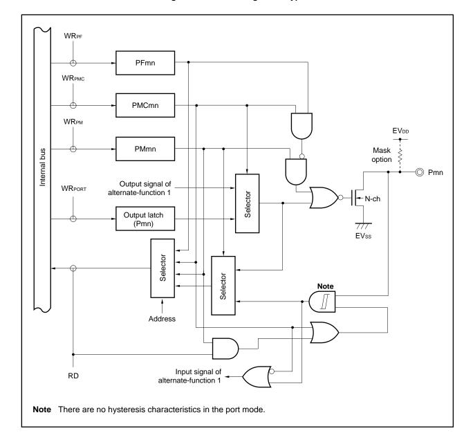
Figure 4-21. Block Diagram of Type K
