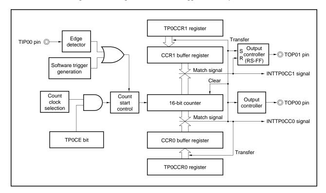
Figure 6-16. Configuration in External Trigger Pulse Output Mode
