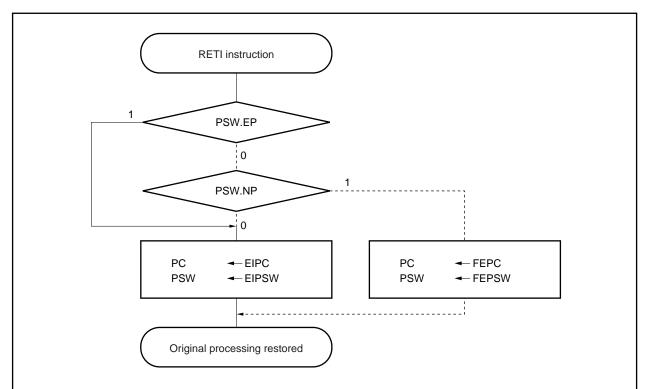
Caution When the EP bit and the NP bit are changed by the LDSR instruction during software exception processing, in order to restore the PC and PSW correctly during restoring by the RETI instruction, it is necessary to set the PSW.EP bit back to 1 using the LDSR instruction immediately before the RETI instruction.
