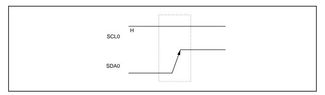
A stop condition is generated when the IICC0.SPT0 bit is set to 1. When the stop condition is detected, the IICS0.SPD0 bit is set to 1 and the interrupt request signal (INTIIC0) is generated when the IICC0.SPIE0 bit is set to 1.
