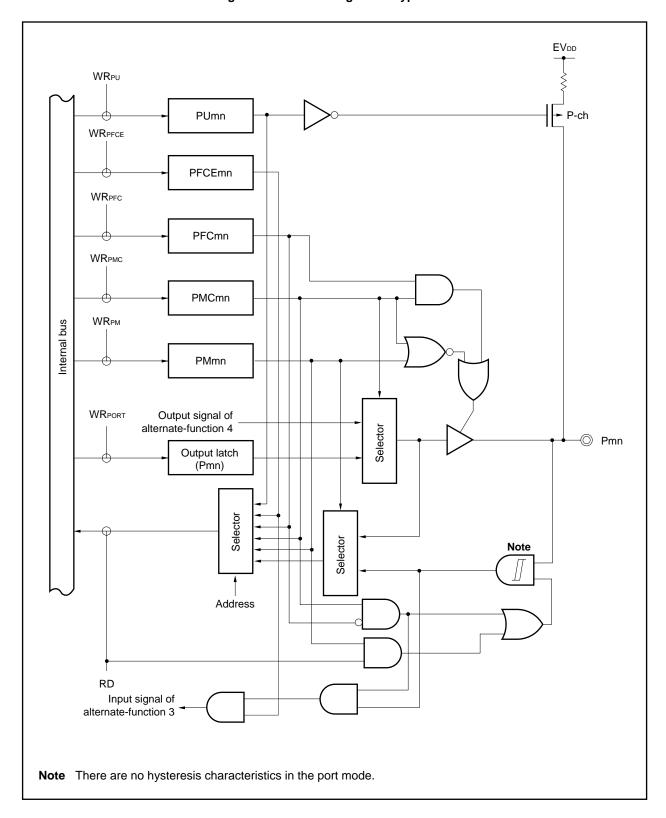
Figure 4-16. Block Diagram of Type G-7-3
