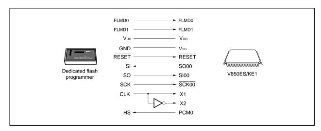
The dedicated flash programmer outputs the transfer clock, and the V850ES/KE1 operates as a slave.
