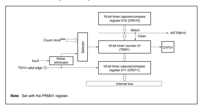
Figure 7-19. Configuration of External Event Counter
