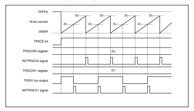
Figure 6-14. Timing Chart When D<sub>01</sub> ≥ D<sub>11</sub>
