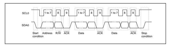
Figure 16-4. I<sup>2</sup>C Bus's Serial Data Transfer Timing
