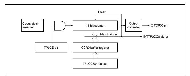
Figure 6-2. Configuration of Interval Timer
