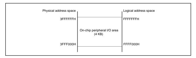
Peripheral I/O registers assigned with functions such as on-chip peripheral I/O operation mode specification and state monitoring are mapped to the on-chip peripheral I/O area. Program fetches are not allowed in this area.
