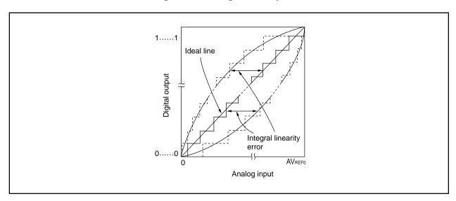
Figure 13-15. Integral Linearity Error
