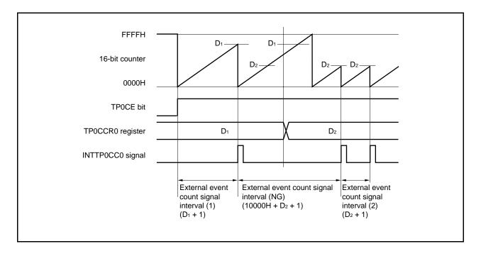
If the value of the TP0CCR0 register is changed from  $D_1$  to  $D_2$  while the count value is greater than  $D_2$  but less than  $D_1$ , the count value is transferred to the CCR0 buffer register as soon as the TP0CCR0 register has been rewritten. Consequently, the value that is compared with the 16-bit counter is  $D_2$ .
