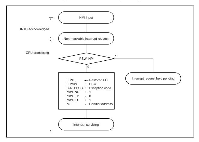
Figure 17-2. Non-Maskable Interrupt Servicing
