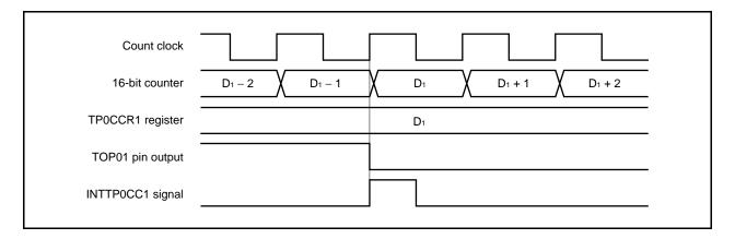
Usually, the INTTP0CC1 signal is generated in synchronization with the next count up, after the count value of the 16-bit counter matches the value of the TP0CCR1 register.
