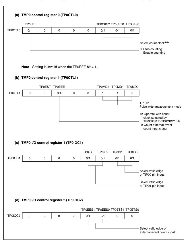
Figure 6-36. Register Setting in Pulse Width Measurement Mode (2/2)
