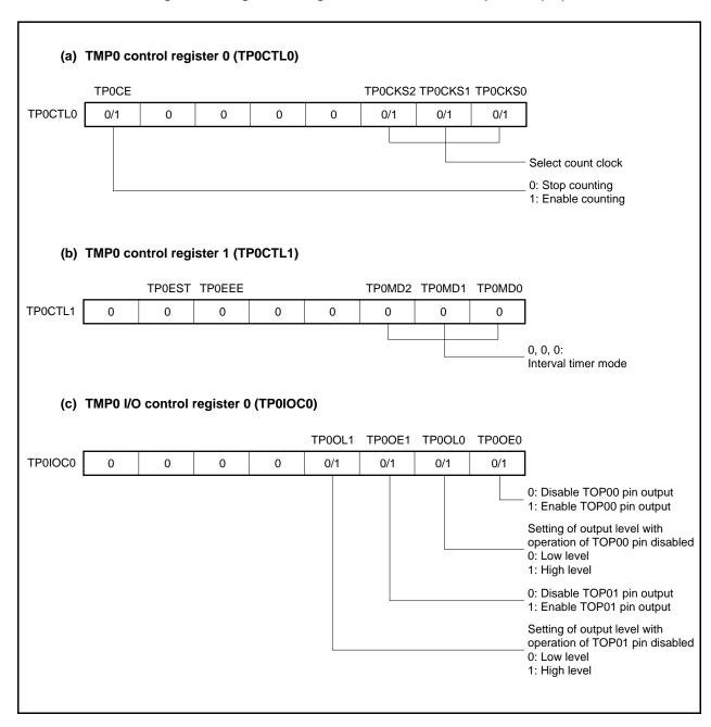
Figure 6-4. Register Setting for Interval Timer Mode Operation (2/2)
