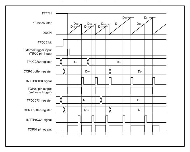
In order to transfer data from the TP0CCRa register to the CCRa buffer register, the TP0CCR1 register must be written.
