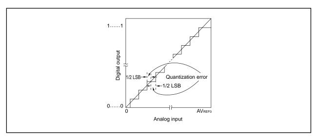
Figure 13-11. Quantization Error
