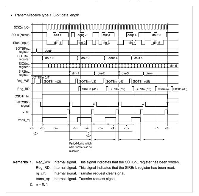
Figure 15-5. Continuous Transfer (Transmission/Reception) Timing Chart
