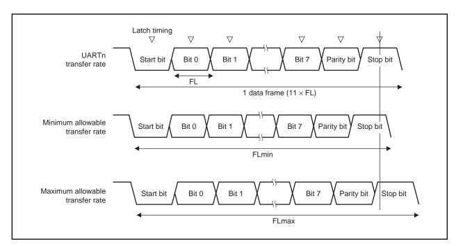
Figure 14-13. Allowable Baud Rate Range During Reception
