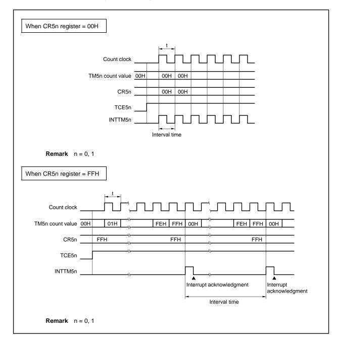
Figure 8-2. Timing of Interval Timer Operation (2/2)
