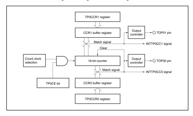
If the set value of the TP0CCR1 register is less than the set value of the TP0CCR0 register, the INTTP0CC1 signal is generated once per cycle. At the same time, the output of the TOP01 pin is inverted. The TOP01 pin outputs a square wave with the same cycle as that output by the TOP00 pin.
