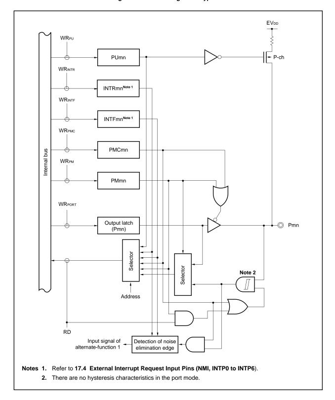
Figure 4-19. Block Diagram of Type H-1
