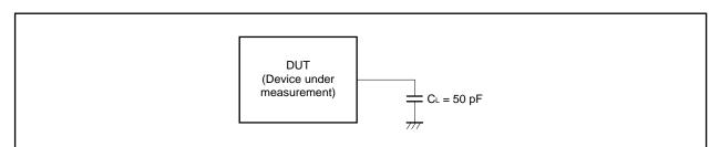
Caution If the load capacitance exceeds 50 pF due to the circuit configuration, bring the load capacitance of the device to 50 pF or less by inserting a buffer or by some other means.
