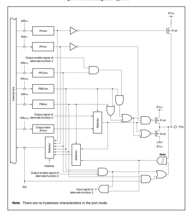
Figure 4-17. Block Diagram of Type G-8
