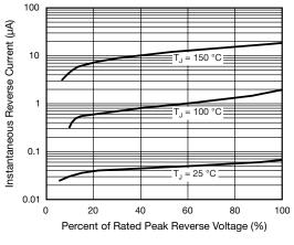
Fig. 4 - Typical Reverse Characteristics
