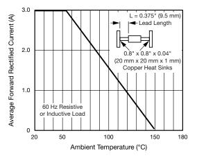
Fig. 1 - Forward Current Derating Curve
