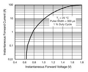
Fig. 3 - Typical Instantaneous Forward Characteristics
