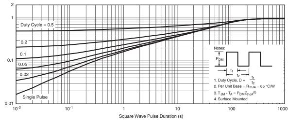
Normalized Thermal Transient Impedance, Junction-to-Ambient
