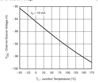
Drain-Source Breakdown vs. Junction Temperature
