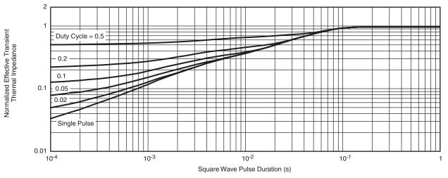
Normalized Thermal Transient Impedance, Junction-to-Case
