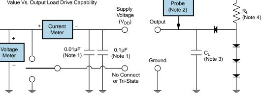
Note 1: An external 0.1µF low frequency tantalum bypass capacitor in parallel with a 0.01µF high frequency ceramic bypass capacitor close to the package ground and V<sub>DD</sub> pin is required.
