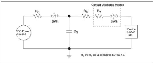
Figure 19. ESD Test Circuit for IEC1000-4-2
