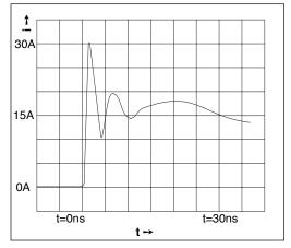
Figure 20. ESD Test Waveform for IEC1000-4-2
