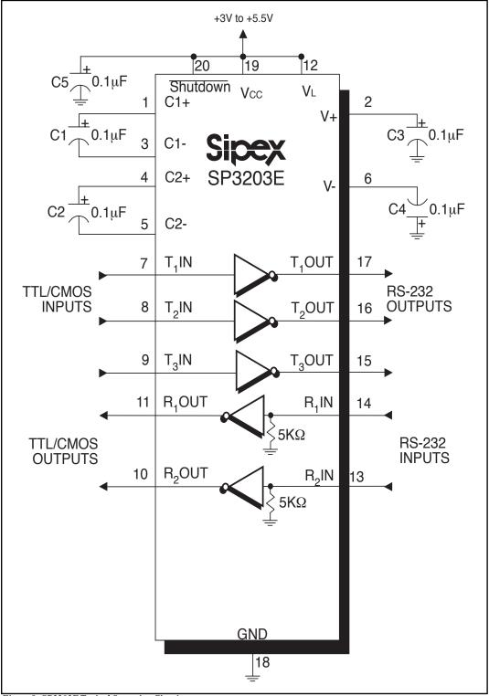
Figure 8. SP3203E Typical Operating Circuit
