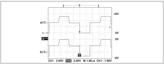
Figure 12. Charge Pump Waveforms
