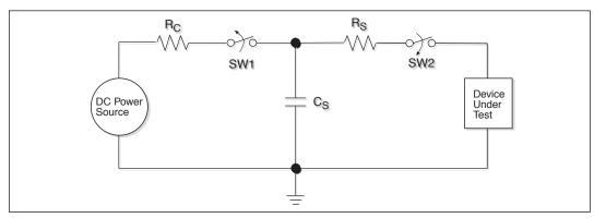
Figure 18. ESD Test Circuit for Human Body Model
