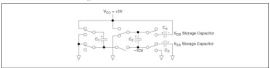
Figure 14. Charge Pump — Phase 3 - V<sub>SS</sub> Charge Transfer
