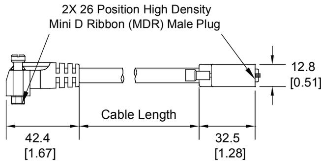
Cable Length Tolerance is the Larger of +50mm / -0mm or +3% / -0%
