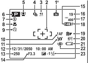
\* In: indicates that no memory card is inserted and that pictures will be stored in the camera's internal memory (pg. 8).
