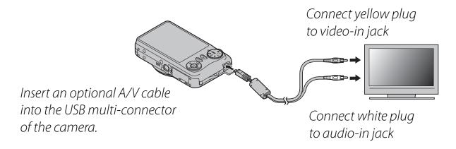
Press for about a second to turn the camera on. The camera monitor turns off and pictures and voice memos are played back on the TV. Note that the camera volume controls have no effect on sounds played on the TV; use the television volume controls to adjust the volume.
