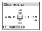
2.1 Press the selector left or right to highlight the year, month, day, hour, or minute and press up or down to change. To change the order in which the year, month, and day are displayed, highlight the date format and press the selector up or down.
