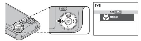
When macro mode is in effect, the camera focuses on subjects near the center of the frame. Use the zoom control to compose pictures.
