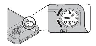
**P (PROGRAM AE)**: Select for control of camera settings such as exposure compensation, white balance, and ISO sensitivity. The mode automatically sets both shutter speed and lens aperture (pg. 20).
