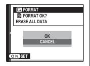
this option will format the memory card. If no memory card is inserted, will be displayed and this option will format internal memory. Highlight **OK** and press **MENU/OK** to begin formatting.
