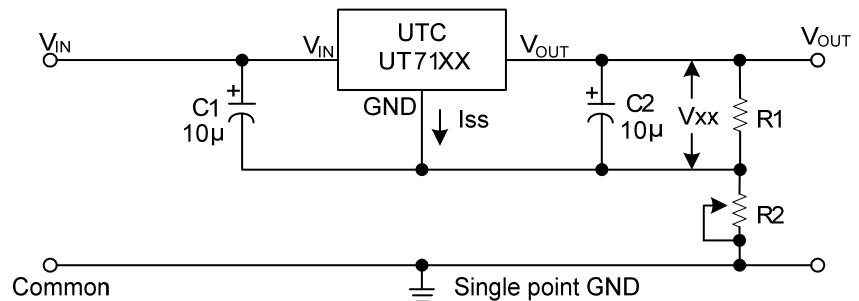
$$\begin{aligned} V_{OUT} &= V_{xx} \left(1 + \frac{R_2}{R_1}\right) + I_{ss} R_2 \\ &\approx V_{xx} \left(1 + \frac{R_2}{R_1}\right) \end{aligned}$$
