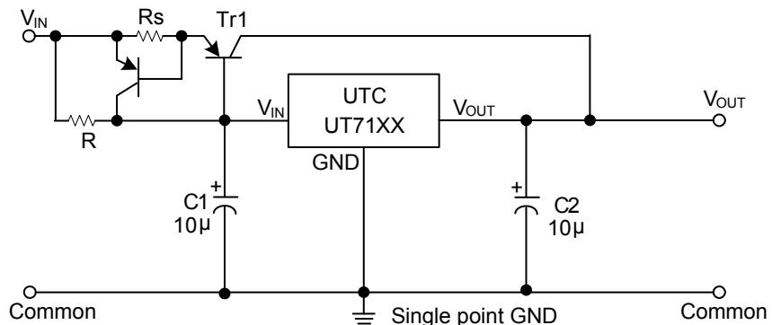
Circuit for increasing output voltage
