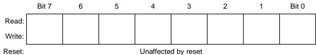
Figure 3-3. Index Register (X)
