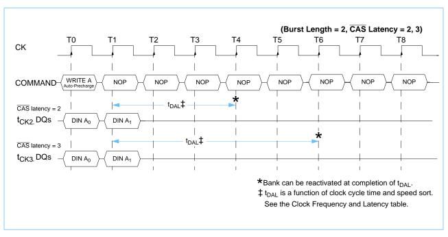
Similar to the Read Command, a Write Command with auto-precharge can not be interrupted by a command to the same bank. It can be interrupted by a Read or Write Command to a different bank, however. The interrupting command will terminate the write. The bank undergoing auto-precharge can not be reactivated until  $t_{DAL}$  is satisfied.
