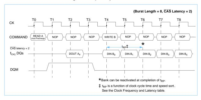
If A10 is high when a Write Command is issued, the Write with Auto-Precharge function is initiated. The bank undergoing auto-precharge cannot be reactivated until t<sub>DAL</sub>, Data-in to Active delay, is satisfied.
