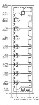
Units: millimeters (inches) Thickness: 0.100 (0.004) (reference only) Chip edge to bond pad dimensions are shown to center of bond pad Chip size tolerance: +/- 0.051 (0.002)
