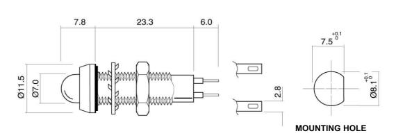
Dimensions in mm (Typical) Not to scale Anode termination indicated by red sleeve Mounting hole to be clean and burr free.
